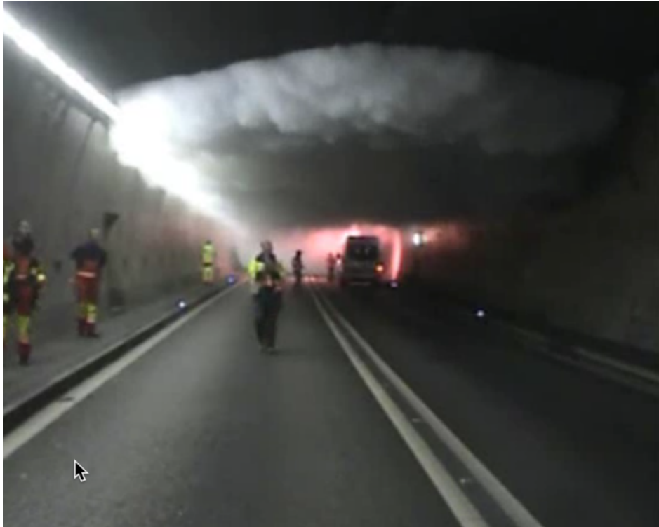
Figure 1. Back layering of smoke at controlled flow conditions
