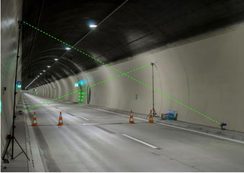
Figure 3. Cross ultrasonic line measurement for calibration of anemometers
